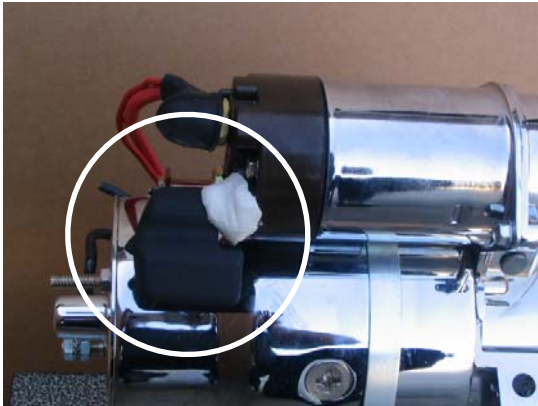
Solenoid Module with Epoxy
