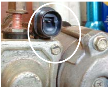
Denso Starter Motors Deutsche Type Ignition Initiate Terminal with Connector Housing Removed.
