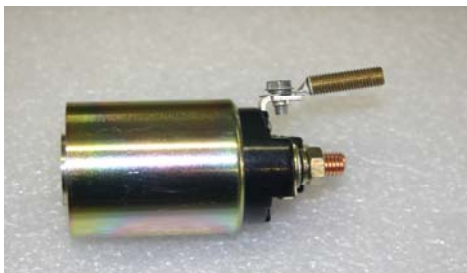
Jeep Solenoid Configuration with Ring Terminal Adapter
