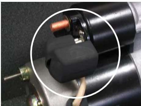
Spade Type Ignition Initiate Terminal with Solenoid Module Attached.
